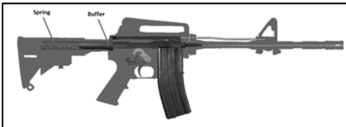
Internal function of an AR-type rifle
